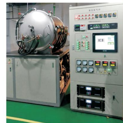
Vacuum Furnace 2500°C 真空炉 2500°C
